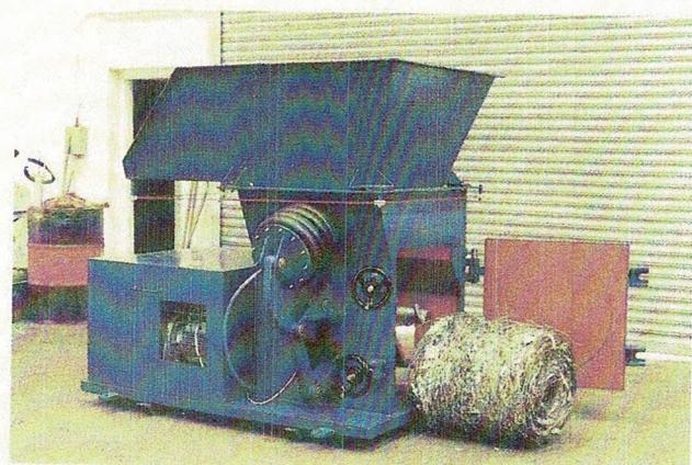
THE LOOSE WIRES ARE FED INTO THE HOPPER AND THEY ARE WOUND ROUND A ROTATING SHAFT. A PRESSURE PLATE AND REDUCER SWITCH REGULATES THE ROLL SIZE AND WHEN OPERATION IS COMPLETE, THE ROLL IS EJECTED BY SIMPLY OPENING THE DOOR AND ROTATING SHAFT IN OPPOSITE DIRECTION. THE 'TS100' CAN BALE WIRE FROM 70-150 PULP BALES INTO COMPACT ROLLS OF CA.500 x 500 MM.
