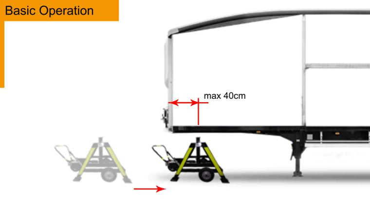
Position the support so that the support beam is fully under the trailer - but no deeper than 40cm from the front.
