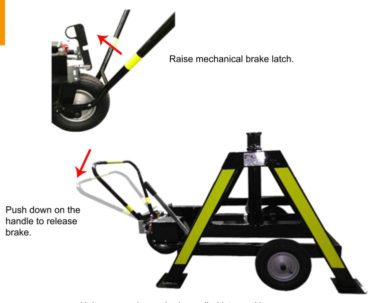
Unit can now be pushed or pulled into position. Releasing the handle will re-apply the brakes automatically.
